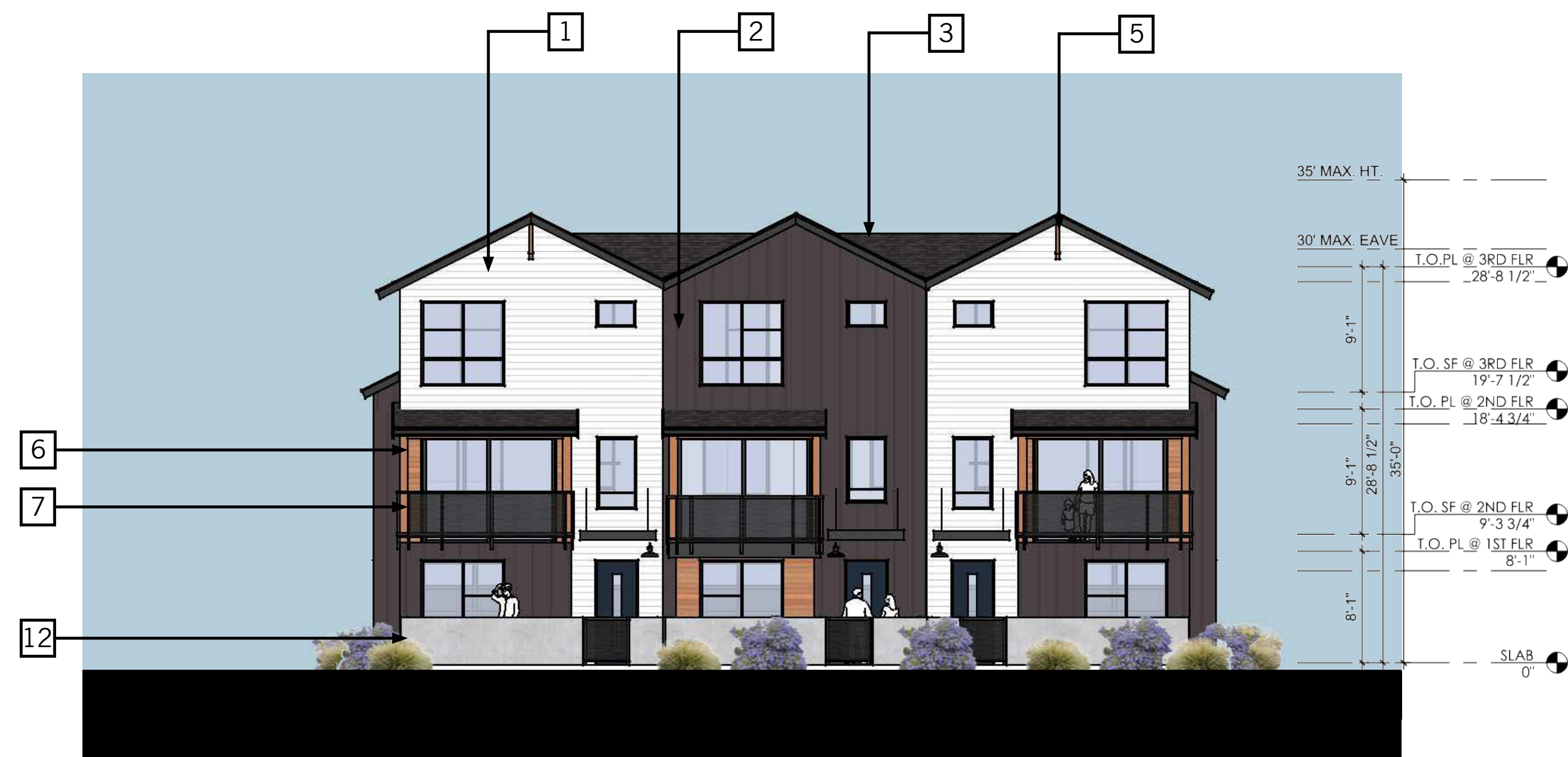
A FRONT EXTERIOR ELEVATION
