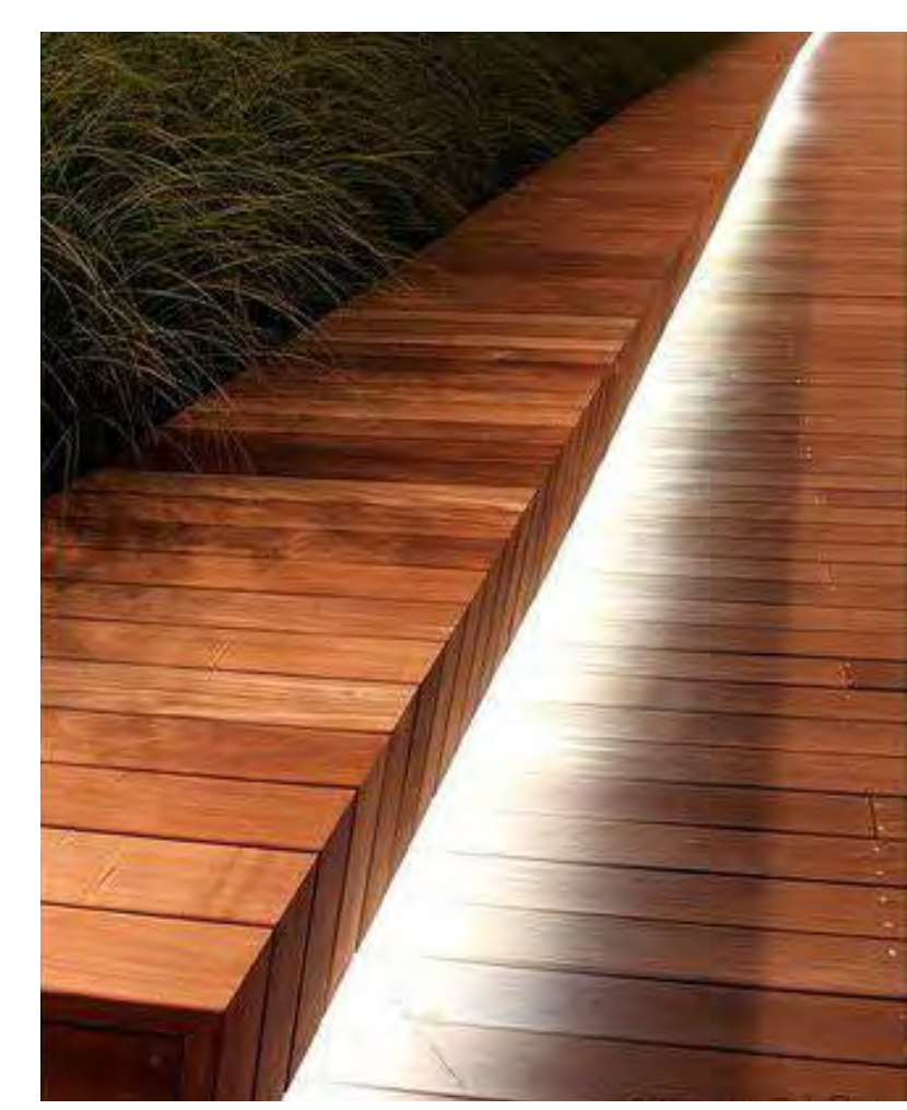
A Linear LED under bench lighting
