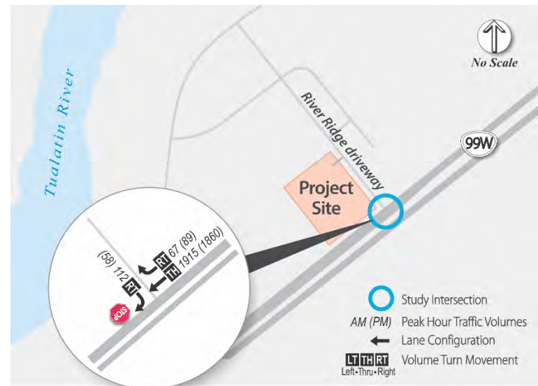
Figure 4: Existing + Project Trips
