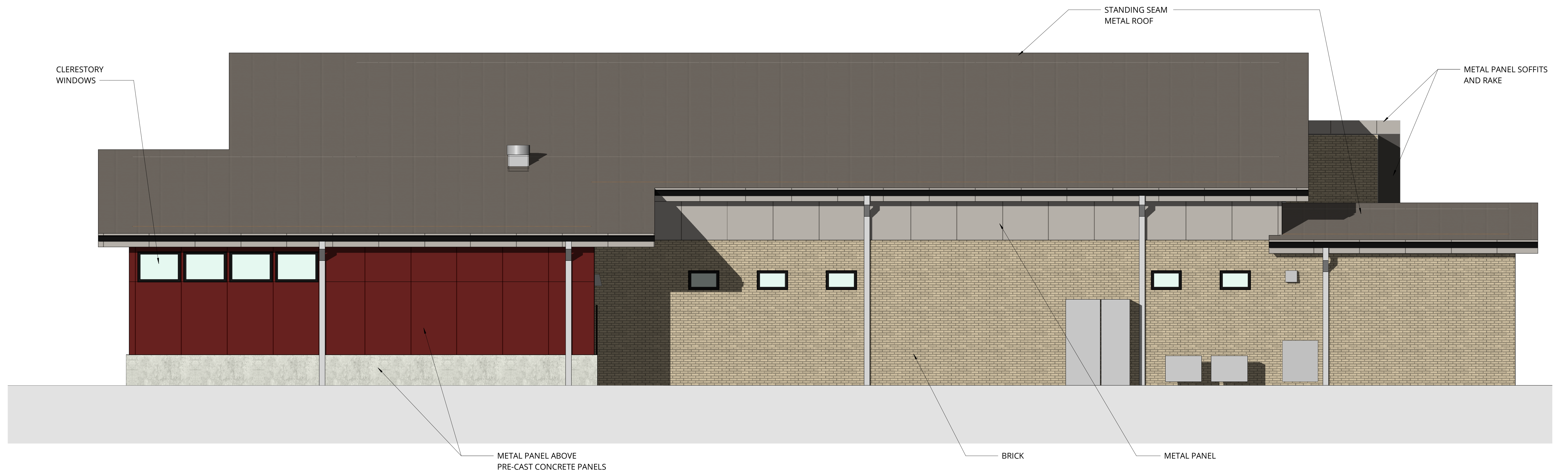
1 NORTH WEST ELEVATION 1/4" = 1'-0"
