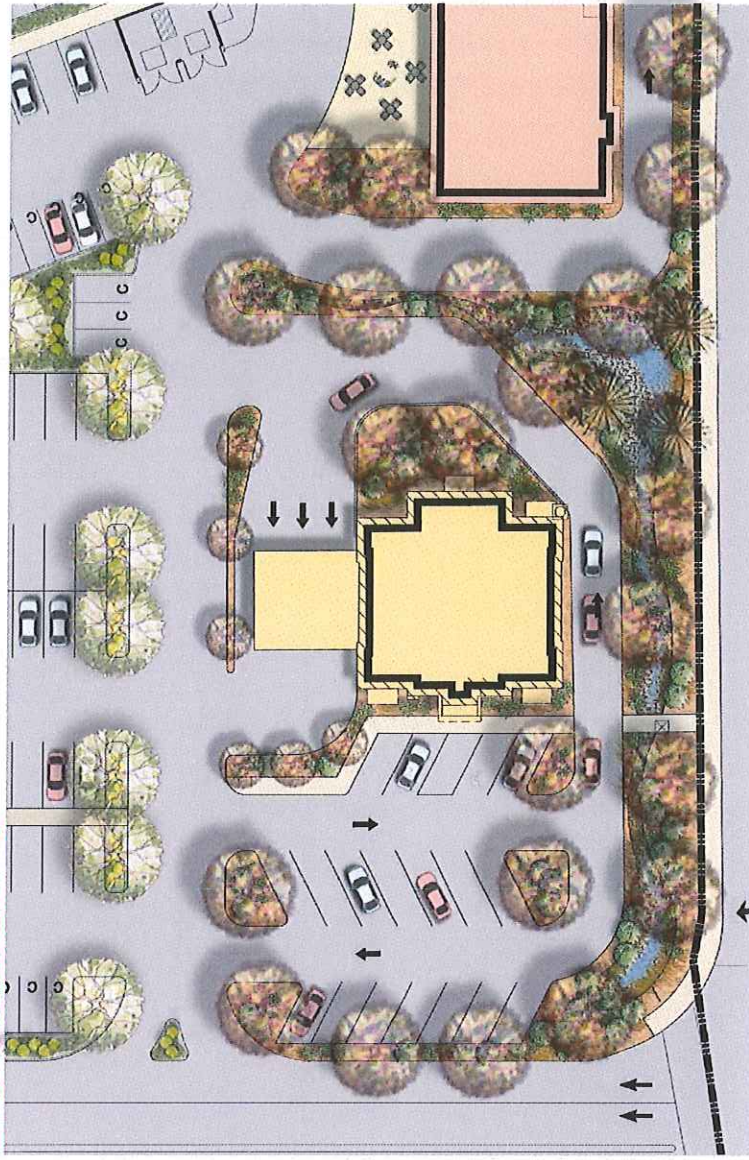
Enlargement 'B' provided conceptual design for a dry creek feature south of Building E-100 and portions along Nyberg Street
