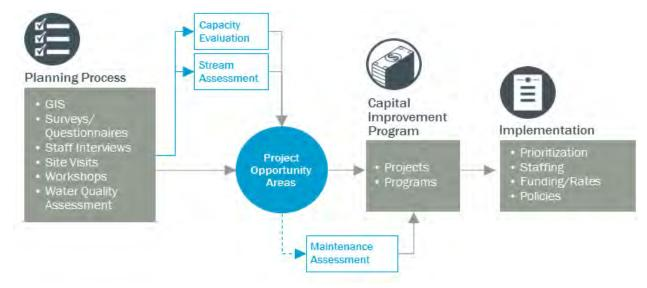
Figure 1-1. Stormwater Master Plan approach
