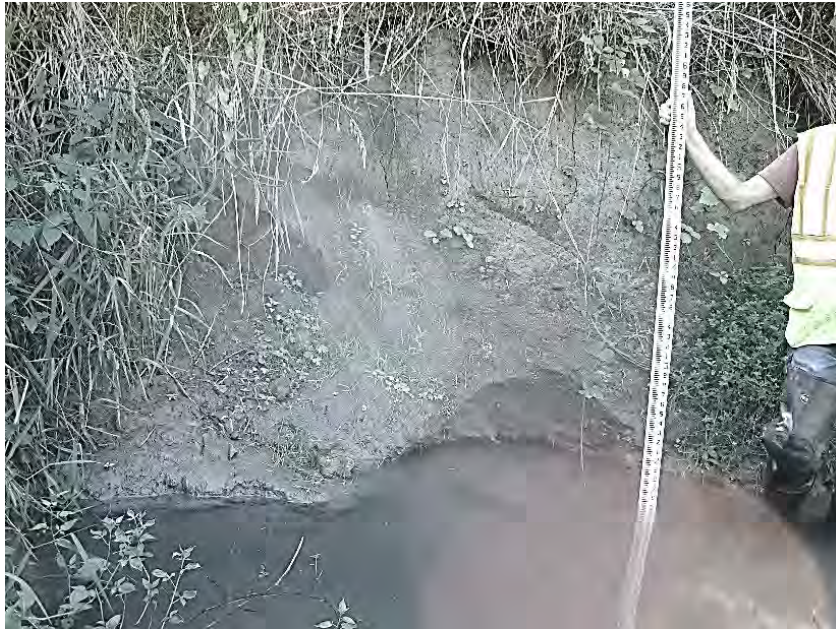
Site location: 150' downstream of SW Borland Rd. Photo number: S1-19 Description: Left bank slump, seepage, wetland plants observed in vicinity
