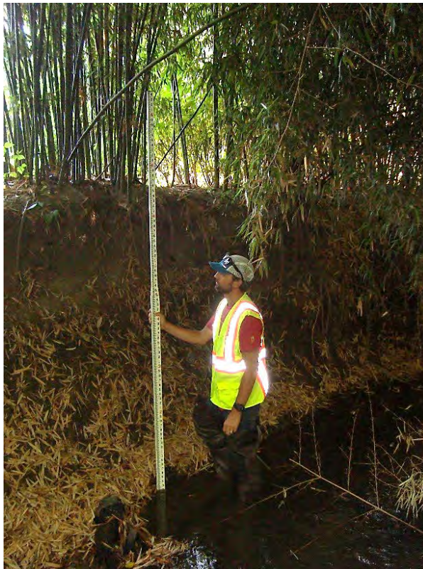
Site location: 30' upstream Photo number: S1-2 Description: 7' high vertical bank (right bank) unstable, bamboo
